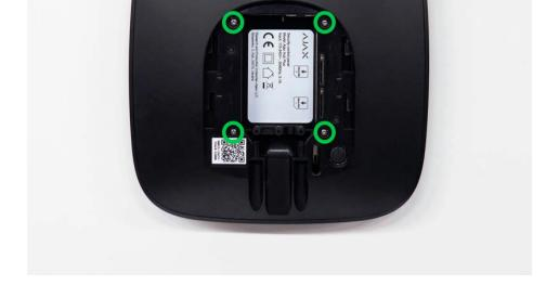
**5.** Remove the screws attaching the boards to the device body.
